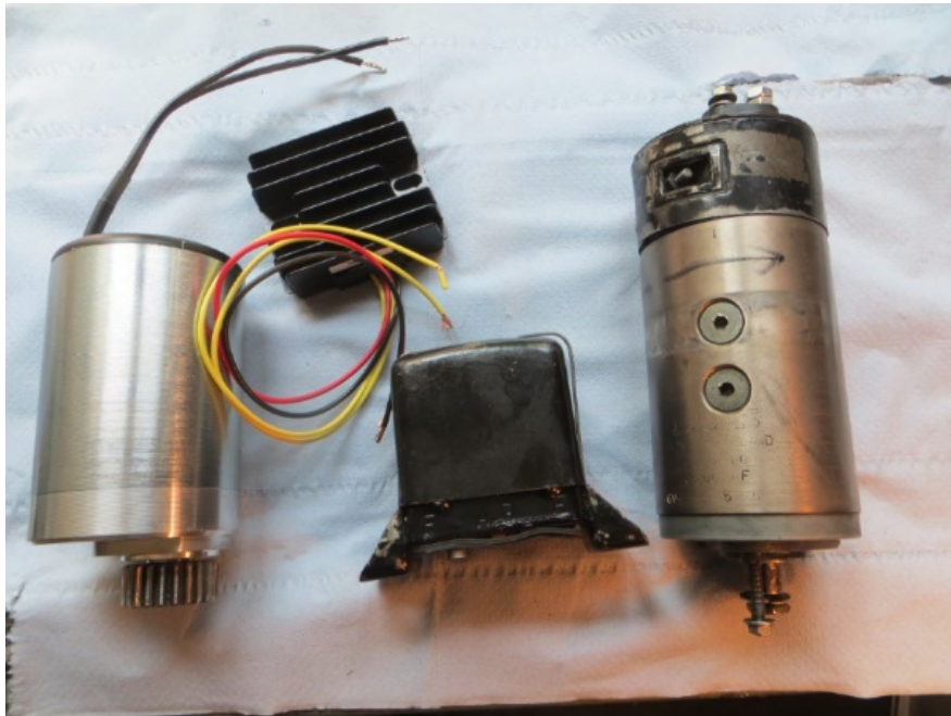
Above: Alton dynamo with electronic regulator against the old 6V system
