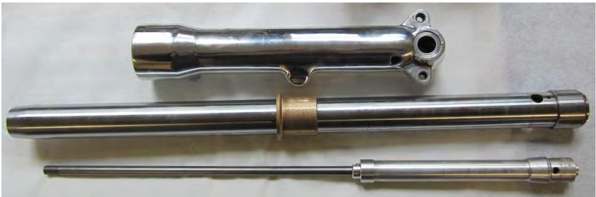
After cleaning the new fork stanchions inside and out- somewhat more careful than we do before we pack them for despatch- applying a bit of oil, fitting new fork bushes, and putting new fibre washers under the damper bodies the bodies are now inserted in the sliders and fastened. Take care to clean the insides of the sliders, too. One finds the sludge of decades in them. Nobody changes fork oil, ever!
