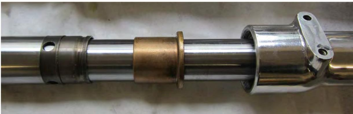
Then, using one of the old top bushes the wrong way round, the fork oil seal can be carefully slide hammered in without damaging it. Now the oil seal holders can be fitted using a strap wrench.
