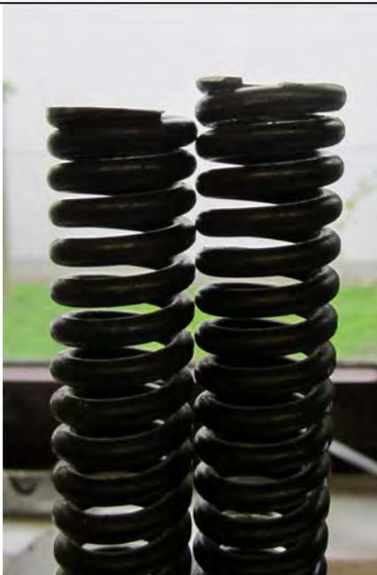
I was about to put the old fork springs back in with a view of test riding them but thought I should check how they compare in length to new ones.
