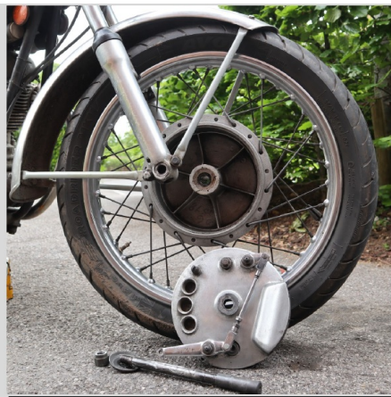
6 Move the wheel forward to release the brake plate assembly
