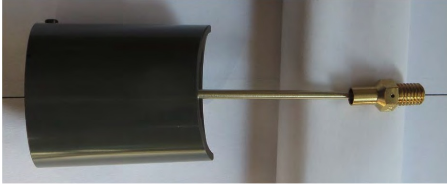
Above: the needle never totally leaves the needle jet which thus is the guide for it.
