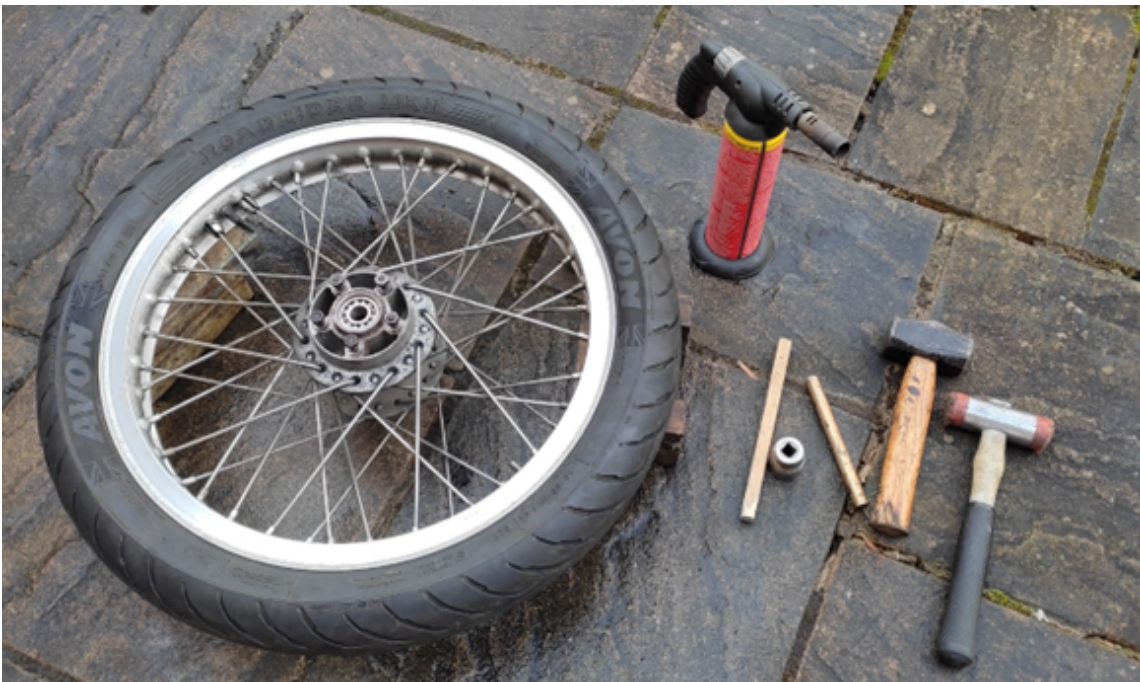
New bearings installed.
