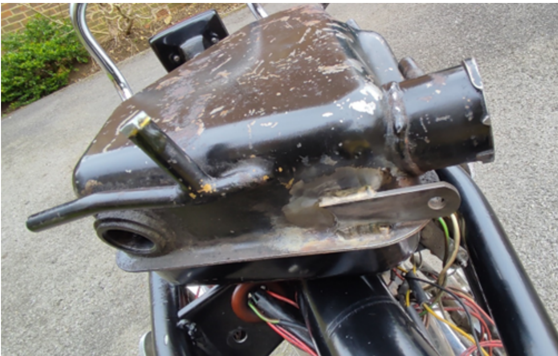
An expertly brazed oil tank bracket.
