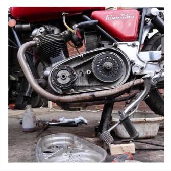
With the cover off & oil drained, I check tension is an easy 3/8", also the condition of the chain. Avoid an overtight chain.
