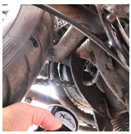
The area around the filter housing is cleaned & a new filter fitted. I refill with 5 pints of Comma 20w50 mineral oil.
