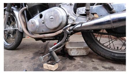
A wooden block under the centre stand leg leans the bike to help drain the oil tank. Left side footrest and brake pedal are removed to access the primary drive cover.
