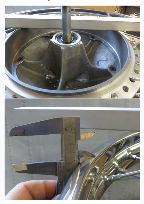
If, as in this case, that dimension is currently wrong I measure where to go with the offset in the bike and re-calculate the distance tube/edge of rim.
