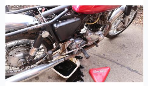
Engine oil is changed annually - irrespective of mileage. The engine sump plug and oil tank drain plug are removed. As usual I spill oil on the drive!
