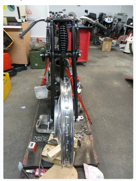
Taking the rim as a given dimension I normally use a straight metal square tube and then measure from a defined plane of the hub down to the outer edge of the rim.
