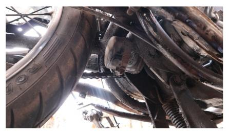
The hose clip securing the filter is corroded and can't be removed with a screwdriver
