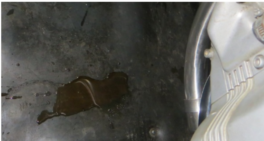
Not, as first thought, a leaking hose, but a small plug in the engine that leaks.
