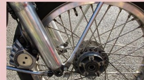
Remove five nuts & washers. Withdraw & replace disc.
