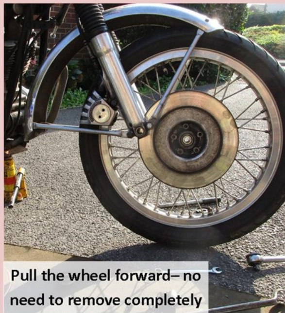
Loosen clamp bolt
