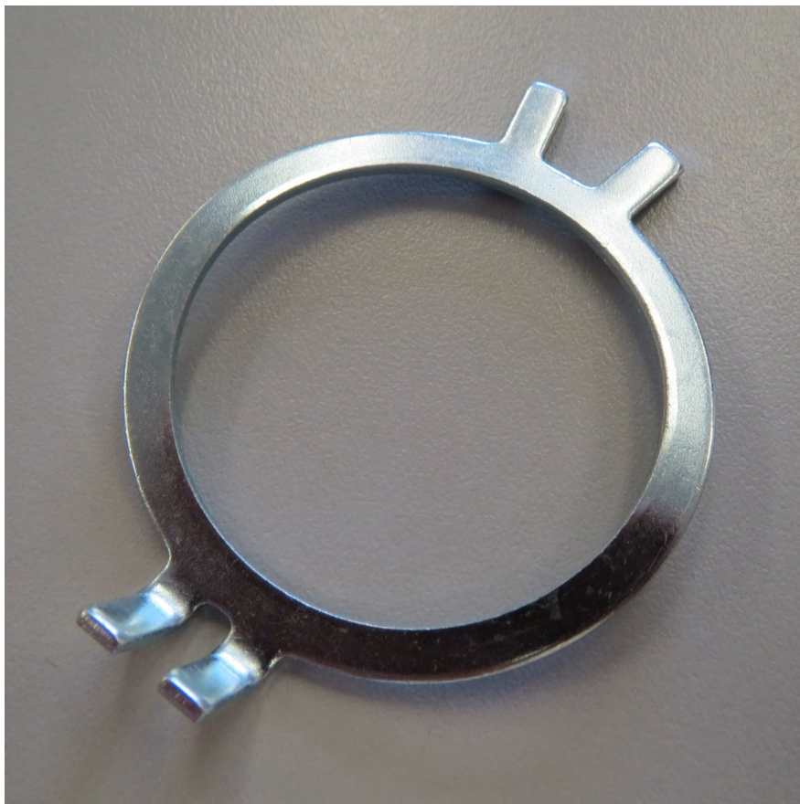
Part# 06.2412. Again, these are only bent into the exhaust locknut with the straight "tongue" when the exhaust pipe has been on for a while and the exhaust nut is in the final position. The bent tongues embrace a cooling fin.
