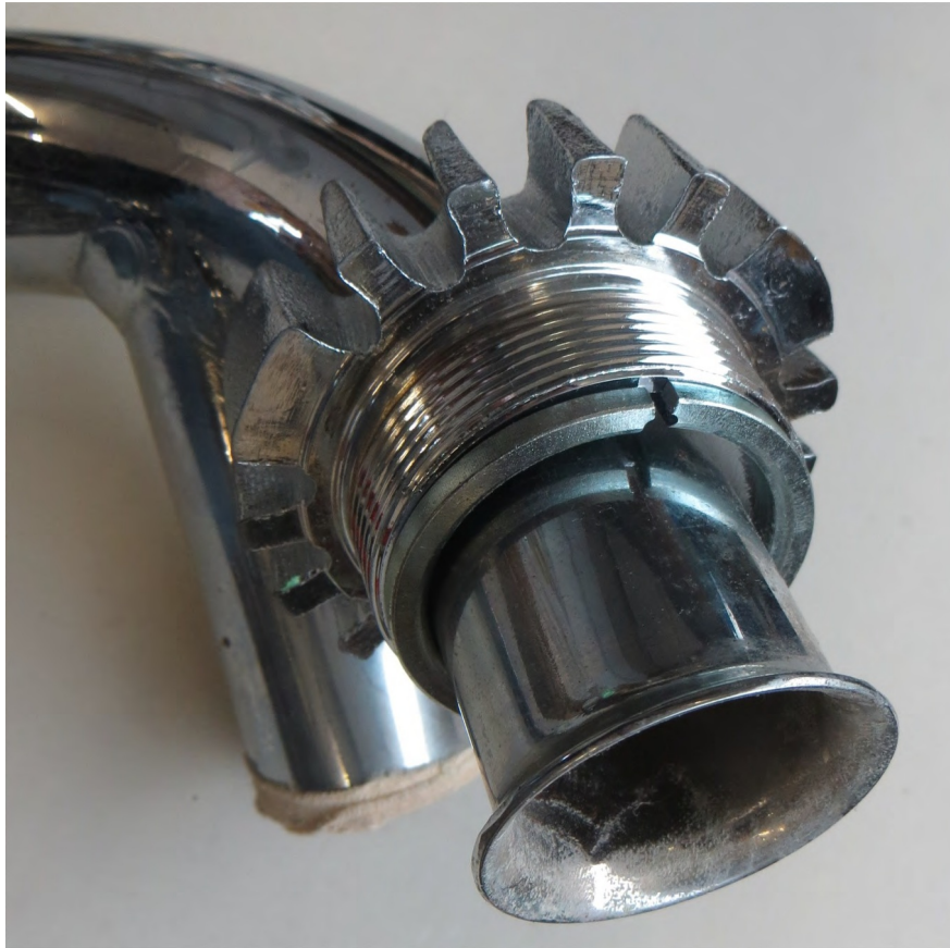
850 exhaust nut (part# 06.3988) and retaining collet (part# 06.5260)
