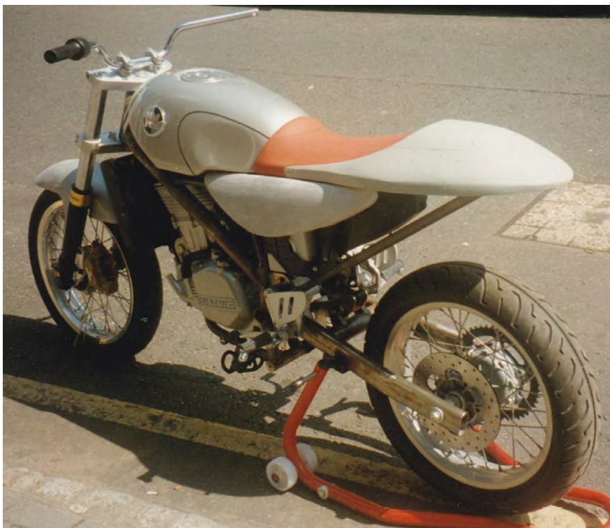
Above: first mock-up with foam seat and side panels, new contour outlined on the petrol tank.
