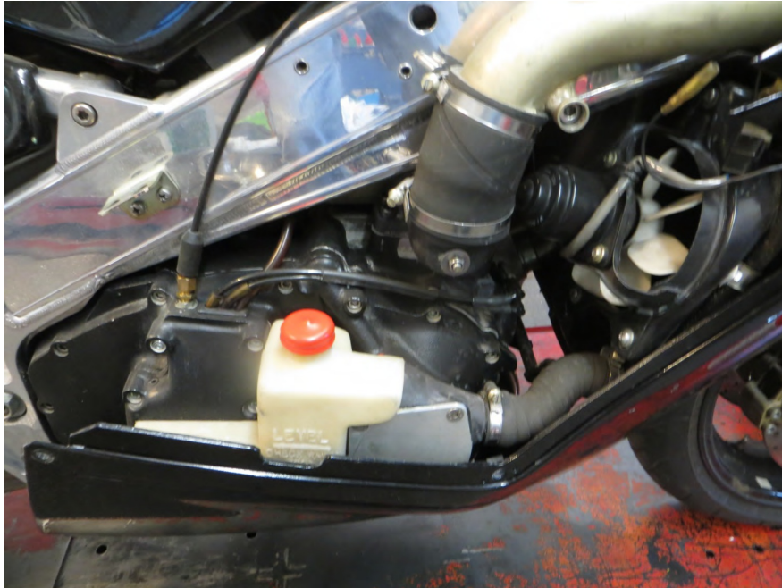
"Lydia" on the workbench. Water pump sits in front of the white plastic tank.
