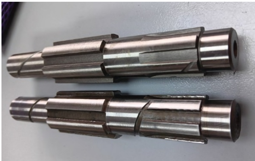
Top our layshaft 06.6666 , bottom something masquerading as a Norton part.
