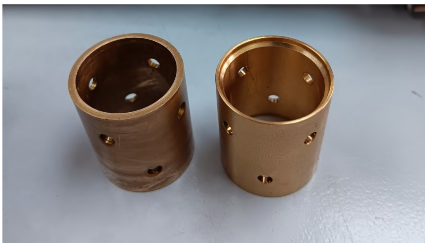
Gear bushes. On the Right ours, at the left, the pirate one.
